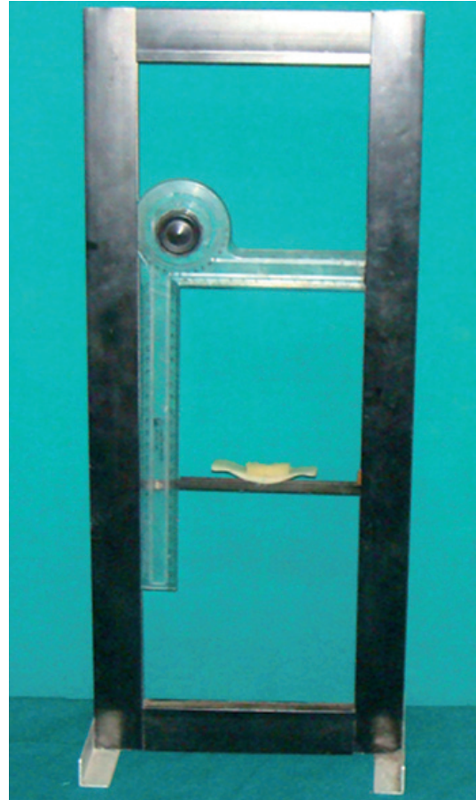
Fig. 1. Modified set square with movable working scales.
