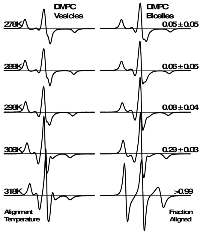
Figure 3. EPR spectra for 5-DSA in DMPC-only vesicles (left) and bicelles (right) as a function of alignment temperature (left text). All samples contain 13% cholesterol (mol cholesterol / mol long-chain lipid). The relative amount of 5-DSA in uniformly oriented bicelles is indicated as fraction aligned (right text).
