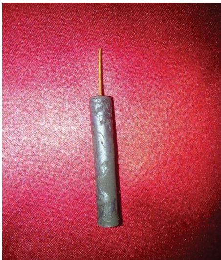
FIGURE 1: Carbon nanotubes paste working electrode.
