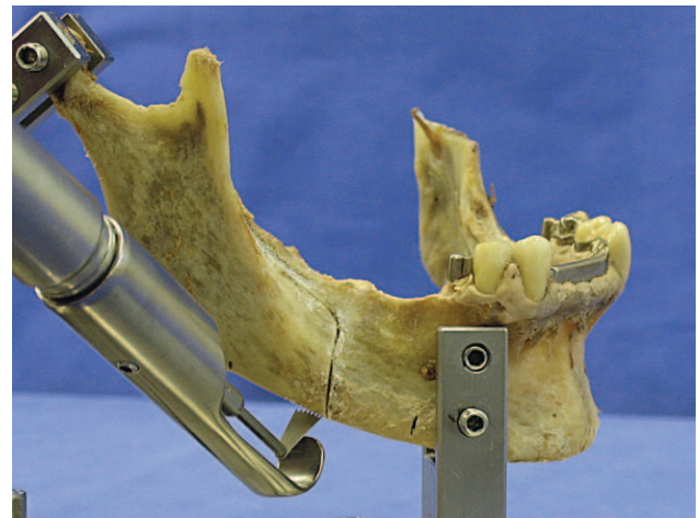
Fig. 5. Buccal view of the fourth osteotomy line in a human mandible mounted on a test rack.
