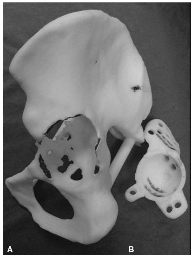
Fig. 2A–B (A) A one-to-one replication of the hemipelvis was created using rapid prototyping technology. (B) The custom acetabular component developed using the model hemipelvis is shown. This component is shown postoperatively in Fig. 3.
