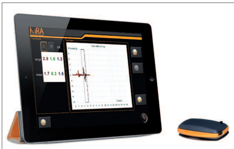
Fig. 1. Graphical representation of the described system (KiRA, Orthokey Ltd, Lewes, Delaware, DE, USA), showing the tablet PC (on the left) running the dedicated acquisition software, and the sensor (on the right). Courtesy of Orthokey Ltd, Lewes, Delaware, DE, USA.
