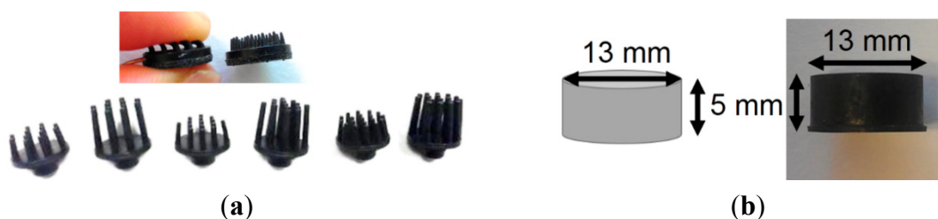
Figure 1. (a) Pin-shaped and (b) cylinder-shaped conductive polymer dry electrodes.
