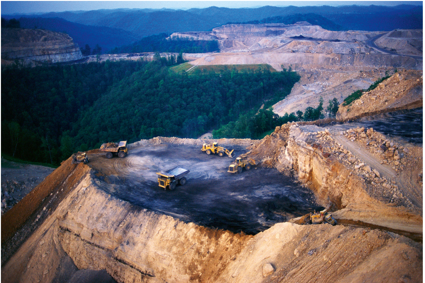
Mountaintop removal strip mining for coal in Appalachia, USA. The mountain tops are blown off and dumped into river valleys in order to get access to the coal layers. It is a particularly destructive form of mining and leaves infertile mesas in what were once diverse temperate forests. - Goerge Steinmetz/Corbis.
