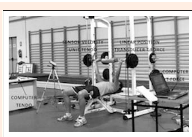
Figure 1. The distribution and location of the TWAS and the TFDMS in the Smith machine, for data acquisition.
