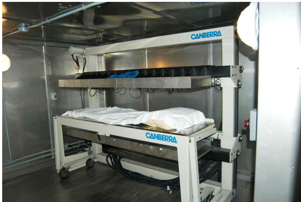
Figure 1. Whole-body K-Counter used in this study at the University of Texas Medical Branch.
