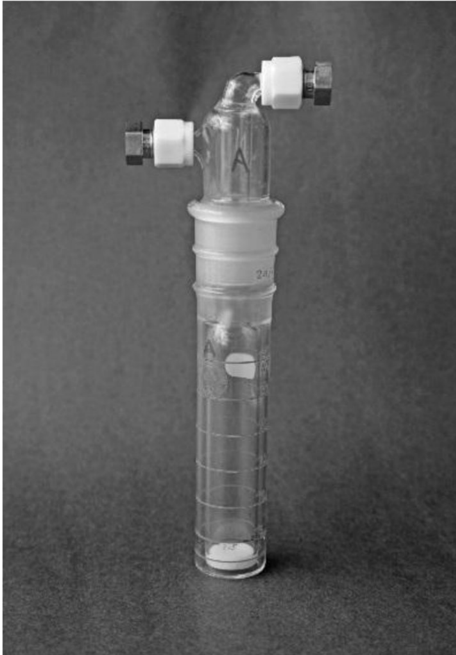
Fig. 2. Custom bubbler required less than 5 mL HD to generated controlled vapor concentrations.
