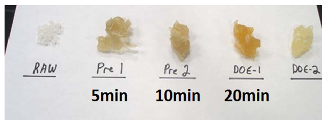
Fig. 3. Effect of processing conditions on PVC resin color: Raw—unprocessed resin; melted, processed resins: for Pre1, Pre 2, DOE-1, bowl temperature=182°C at labeled mixing times; for DOE-2 bowl temperature=192°C for 5 min with nitrogen purge
