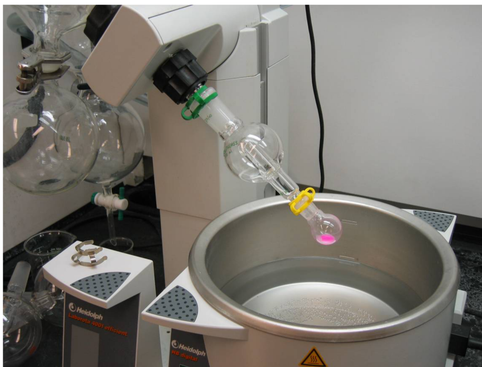
Fig. 2. Remove chloroform by rotary evaporation.
