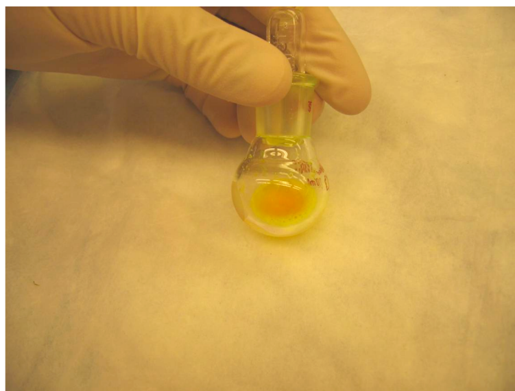
Fig. 4. The thin lipid film (red) at the bottom of the flask is completely dispersed in the buffer containing 2 mM HPTS (green).
