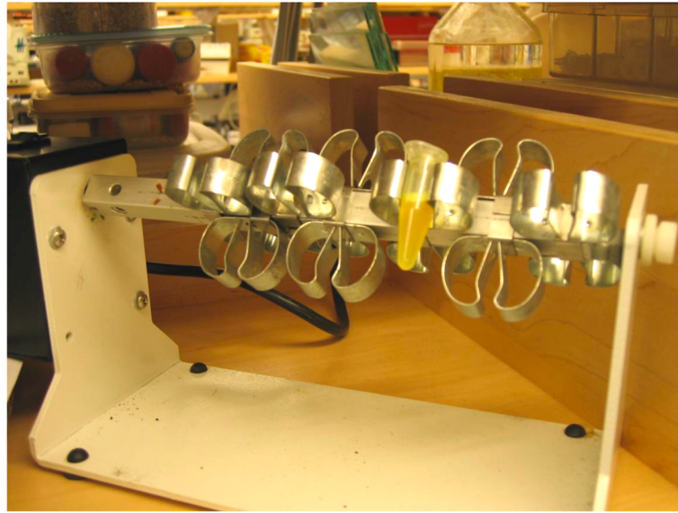
Fig. 5. Vesicle suspension in a 1.5 ml Eppendorf tube, on a bench top rotary tumbler.
