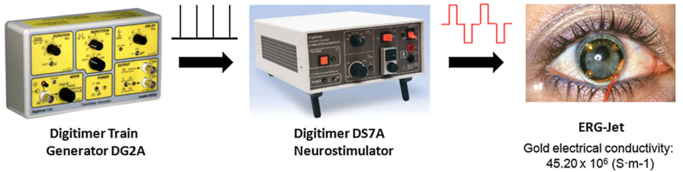
Fig. 2. Neurostimulator setup for TcES. Digitimer train generator (DG2A) generates the pulse triggers for the Digitimer DS7A neurostimulator which in turn outputs alternating polarity current pulses to the ERG-Jet electrode (photograph courtesy of Fabrinal SA).
