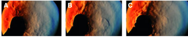
Figure 2. Examples of Schlieren images of an 80 year-old man, whilst coughing without wearing any mask (A), whilst wearing a surgical mask (B) and whilst wearing an N95 mask (C). (All images by Thomas J Liebner and Gary S. Settles).
