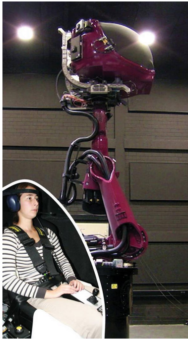
Fig. 1 Experimental set-up. Participants sat inside the simulator's cabin, where visual stimuli were presented on the inner surface of the cabin door by means of two projectors (stimulus resolution: 19.6 px/deg, refresh rate: 60 Hz, FOV: 70 × 90 deg)
