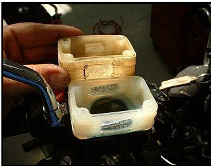
Figure 2 A plastic item with thirty years of exposure to heat and cold, brake fluid, and sunlight.
