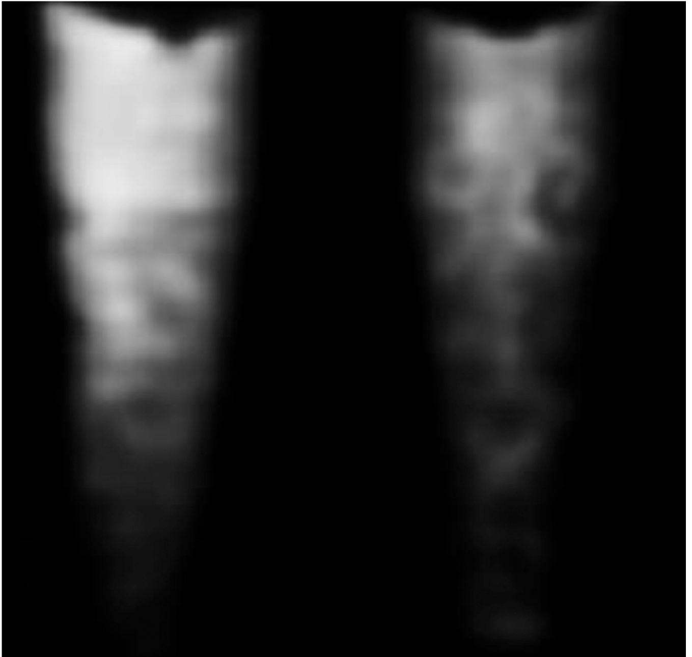
Figure 4. SFHI x-ray scatter image of FOCUS cells incubated with 10 nm SPION-COOH-PAH at 20 ppm (left) and FOCUS cells without SPIONs (right).
