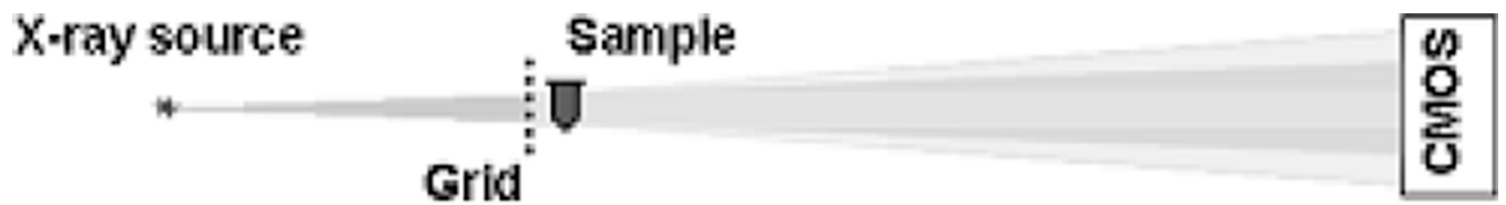
Figure 1. Schematic of the x-ray imaging setup.
