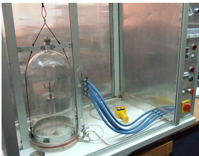
Fig. 1 Cold plasma generator
