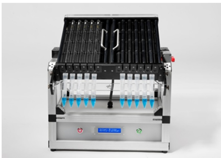
Figure 2 Pipette-Clinostat developed at DLR (Design: Jens Hauslage).
