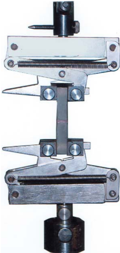
FIGURE 3- Tensile strength specimen in the universal testing machine
