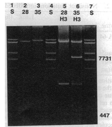
FIG. 4. Twenty-eight-kilobase and 35-kb products without (lanes 2 and 3) and with (lanes 5 and 6) digestion by Hind III. Before Hind III digestion, the 28-kb product was amplified with 21 min of extension time per cycle, and the 35-kb product was cycled with 24-min extension times, both in the RoboCycler at optimum pH. Lanes S (1, 4, and 7) contained undigested and Hind III-digested \lambda plac5 DNA.
