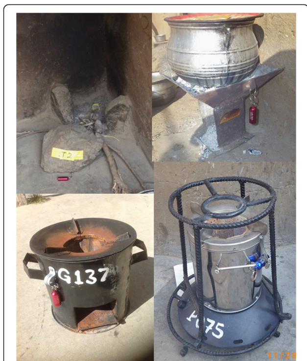
Figure 4 Traditional and improved stove technologies being compared in the REACTING study, shown with Stove Use Monitors (SUMs) attached. Top left: traditional three-stone stove. Top right: traditional charcoal stove. Bottom left: Philips Smokeless Stove, Made in Lesotho (Southern Africa), Cost: ~US$125. Bottom right: Gyapa Wood-Burning Stove. Made in Accra. Cost: ~US$15-25.
