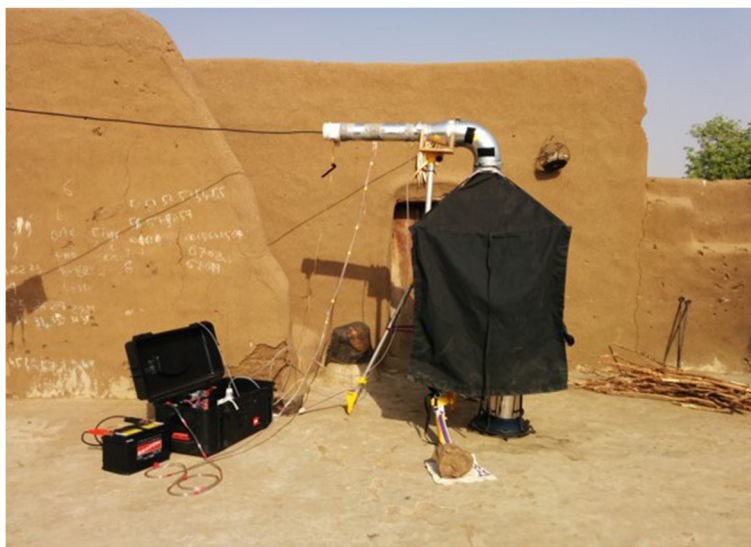
Figure 5 E-Pod setup for measuring in-field stove emissions.
