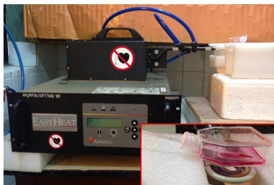
Figure 1 Hot Shot System 2 radiofrequency generator attached to a pancake-shaped coil. The pancake-shaped coil used for the temperature rise in the cell culture flask is magnified in the inset.
