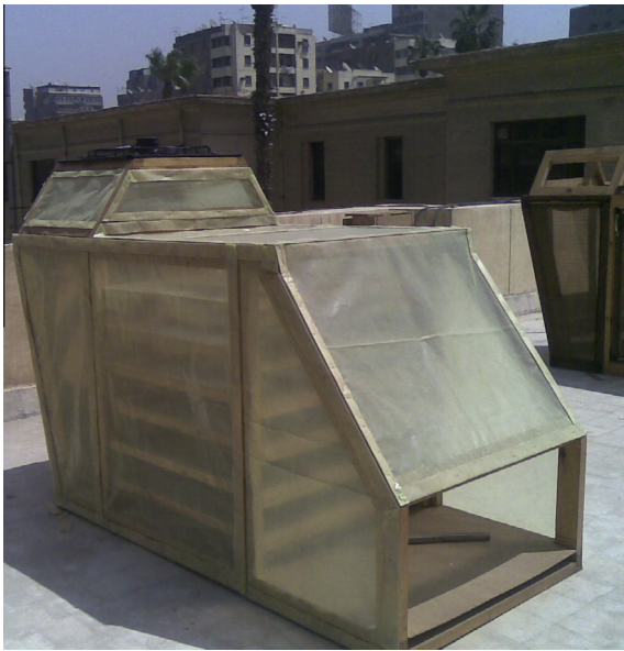
Fig. 2 Photograph of the direct solar dryer.
