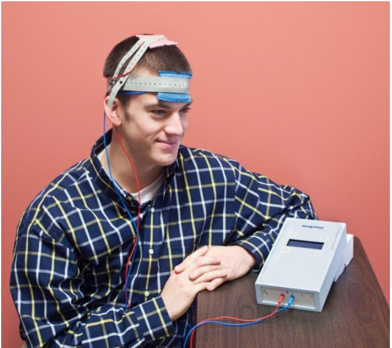
Fig. 1. This is a mock depiction of the tDCS delivery. The salmon-colored electrode is the anode, or excitatory electrode; it was placed over the cortical motor area controlling the lower extremity. The blue electrode is the cathode, or inhibitory electrode; it was placed supraorbitally.
