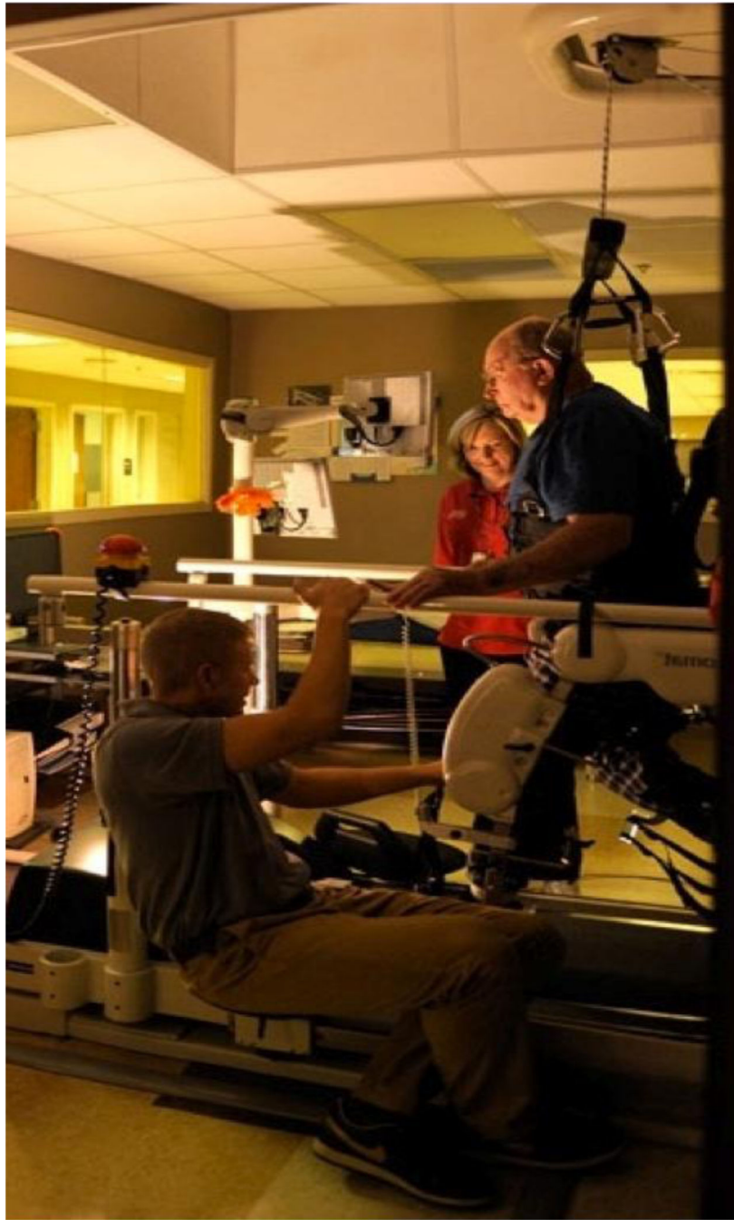
Fig. 2. LT-RGO (Lokomat, Hocoma Inc, Switzerland). The harness system provides body weight support. The robotic exoskeleton facilitates a bilaterally symmetrical gait pattern as the user attempts to walk on the treadmill.
