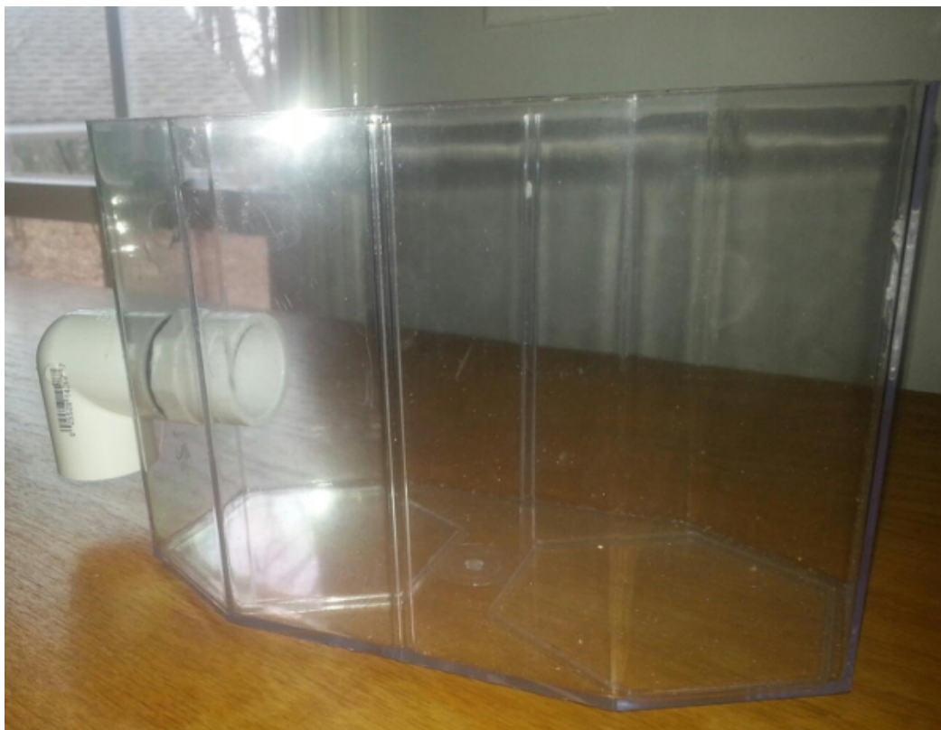
Figure 6: Representative fish tank. The fish tank contains a draining line that will connect with the horizontal draining lines in the system.
