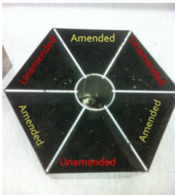
Figure 1. Earthworm avoidance wheel. The wheels are produced from steel and the worms are allowed to move throughout the compartments via multiple holes which are approximately 5 cm in diameter.
