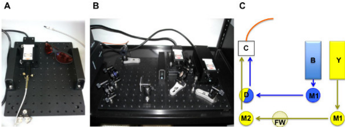
Figure 2. Laser systems used for in vivo optogenetic stimulation. (A) Single laser system for in vivo stimulation. This laser is physically pre-coupled by manufacturer and requires little end user set-up. (B) Dual laser system. Two lasers are coupled into a single fiber through the use of mirrors that act to steer each beam path into a non-contact style coupler. This is the most versatile set-up as optical components can be removed or added as needed but presents more of a challenge in terms of efficient laser coupling. (C) Schematic of dual laser system shown in (B) indicating placement of lasers and mirrors with the corresponding laser light beam path (arrows) depicted. Here, the dichroic mirror “D” is used to deflect blue wavelengths of light while transmitting yellow wavelengths through to the coupler “C” and into the attached coupler patch cord. B = blue laser; C = non-contact style coupler; D = dichroic mirror; FW = filter wheel; M = Mirror; Y = yellow laser. Please click here to view a larger version of this figure.
