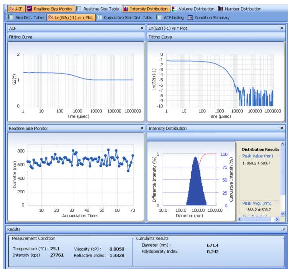
Figure 1. Analysis screen shot showing dynamic light scattering measurement of particle size. The top two panels show the plots of the autocorrelation function, G_2(\tau) , and logarithm of [G_2(\tau)-1] over time. The instrument's digital signal processor (correlator) expresses the detected light intensity as a function of delay time ( \tau ). The plot shows that SDF-1 \alpha -DS-CS particles caused an exponential decay of the intensity between 0.2-2 msec. To obtain the average decay constant \langle \Gamma \rangle , a program analyzes the \text{Ln}[G_2(\tau)-1] plot with cumulants fitting. The first order coefficient of the derived polynomial equation is assigned to \langle \Gamma \rangle , which is proportional to the slope of the curve. The second order coefficient divided by the square of \langle \Gamma \rangle is the polydispersity index, which describes the intensity distribution width. From \langle \Gamma \rangle the average diffusion coefficient ( \langle D \rangle ) and particle diameter ( d ) are calculated as: \Gamma = D \cdot q and D = k_B T / 3\pi\eta_0 d (Stoke-Einstein equation). The middle two panels show the fluctuation of the size reading during the 70 accumulation measurements, and the size distribution calculated with respect to intensity in the measurement. The cumulants diameter and polydispersity index are shown at the bottom of the screen.
