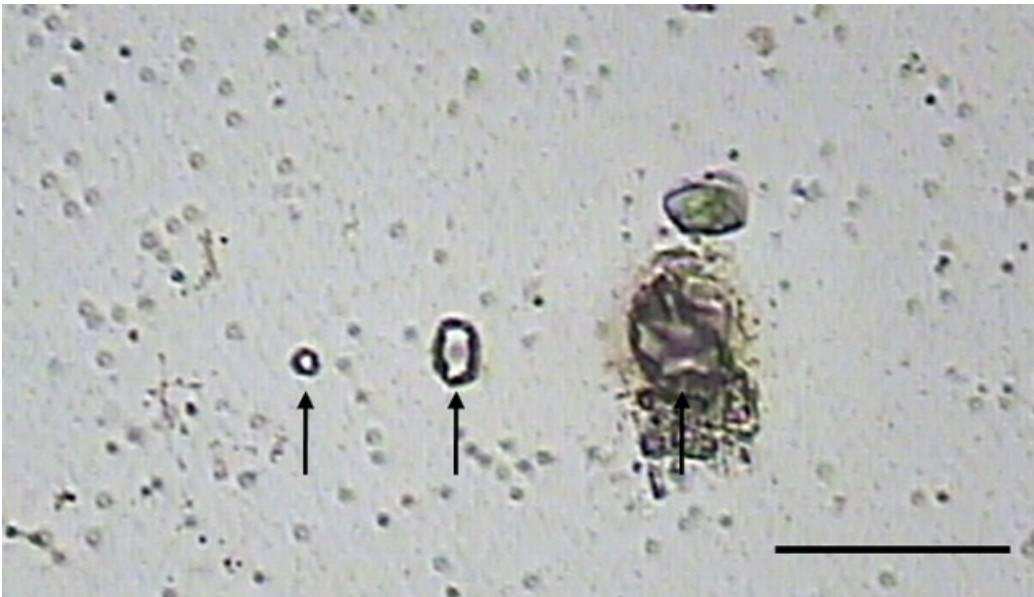
Figure 5. Using the UV cutting laser. The UV cutting laser is used to cut through the PEN membrane and tissue. Prior to use the minimum intensity needed to cut through the membrane and tissue needs to be determined since the UV laser can damage tissue. Above, the three spots (Arrows) of different UV laser intensities are shown with the left spot size sufficient for 10 \mu m sections, the middle spot for thicker sections and the right spot demonstrating a UV laser intensity that is too high. Scale bar = 100 \mu m. Please click here to view a larger version of this figure.
