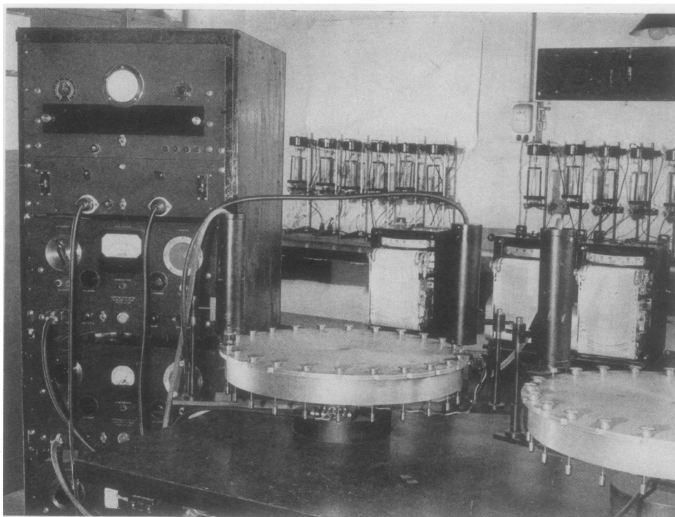
FIG. 5. APPARATUS FOR MEASURING THE RADIOACTIVITY OF Fe^{55} AND Fe^{59} SAMPLES
