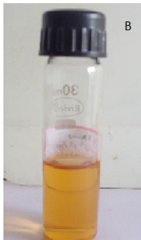
Fig. 1 Ag nanoparticle solutions, synthesized by reducing \text{AgNO}_3 using Vasaka leaf extract
