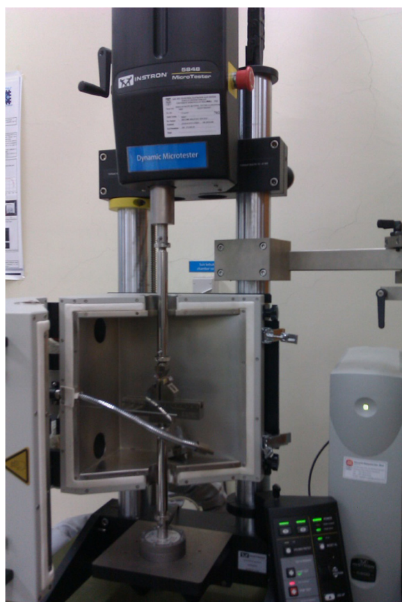
Figure 1 Instron Universal Microtester.
