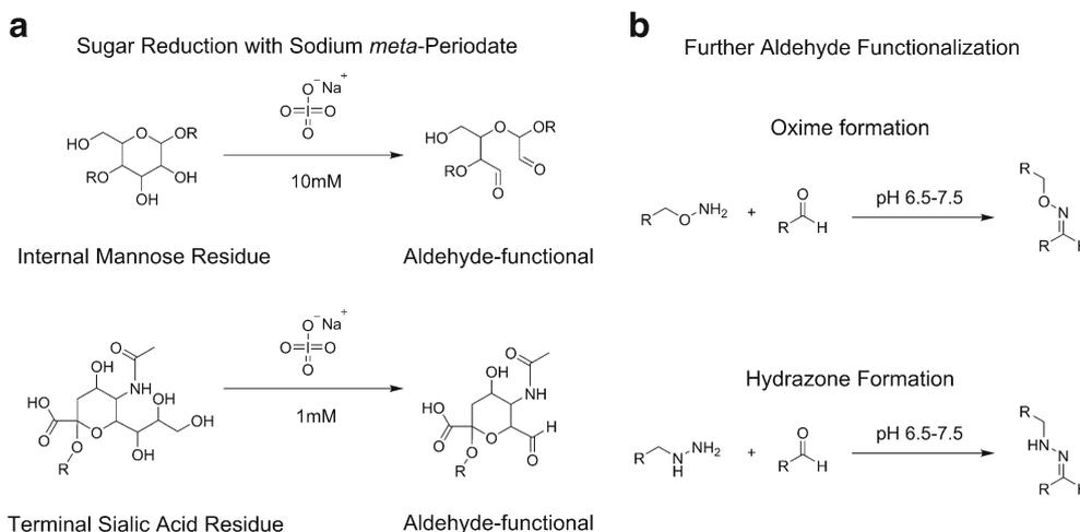
**Fig. 6.** Native sugars in the glycosylated sites of antibodies can be conjugated to functional linkers in a two-step process: **a** internal mannose or terminal sialic acid residues are reduced to aldehydes and **b** aldehydes react with linkers containing hydroxylamine or hydrazines to produce oxime and hydrazones, respectively
