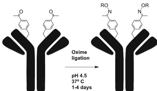
**Fig. 3.** Site-specific conjugation of alkoxy-amine-derivatized auristatin to anti-Her2 Fab and IgG with pAcPhe. The IgG is coupled by oxime ligation to drug derivitized with a terminal alkoxy-amine through pAcPhe residues (adapted from *Proc. Natl. Acad. Sci. U. S. A.* 109, 16101–6)
