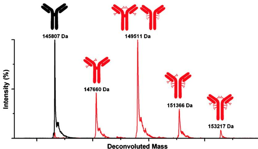
**Fig. 9.** ESI-MS is used to produce these deconvoluted mass spectra of a deglycosylated ADC in red. The ADC mixture of six different species in red is compared to that of the unconjugated mAb in black (reprinted with permission from *Anal. Chem.* 84, 2843–2849. Copyright 2012 American Chemical Society)
