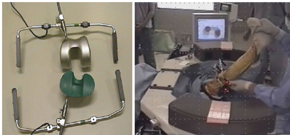
Fig. 7 Photometric system of measurement. The position of all LEDs were detected in three-dimensions by two sets of three linear CCD cameras
