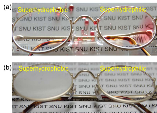
Figure 4 | Superhydrophobic and superhydrophilic lenses in eyeglasses with (a) water spray test on glass surfaces and (b) the condensation test by an incident temperature increase from -17 to 25^{\circ}\text{C} . CF 4 plasma etching duration for both glasses was fixed at 30 min.
