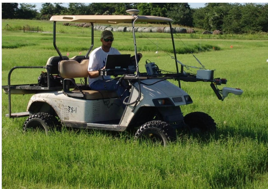
Figure 2. Electric golf cart used for transport of sensors across alfalfa-bermudagrass experiment.
