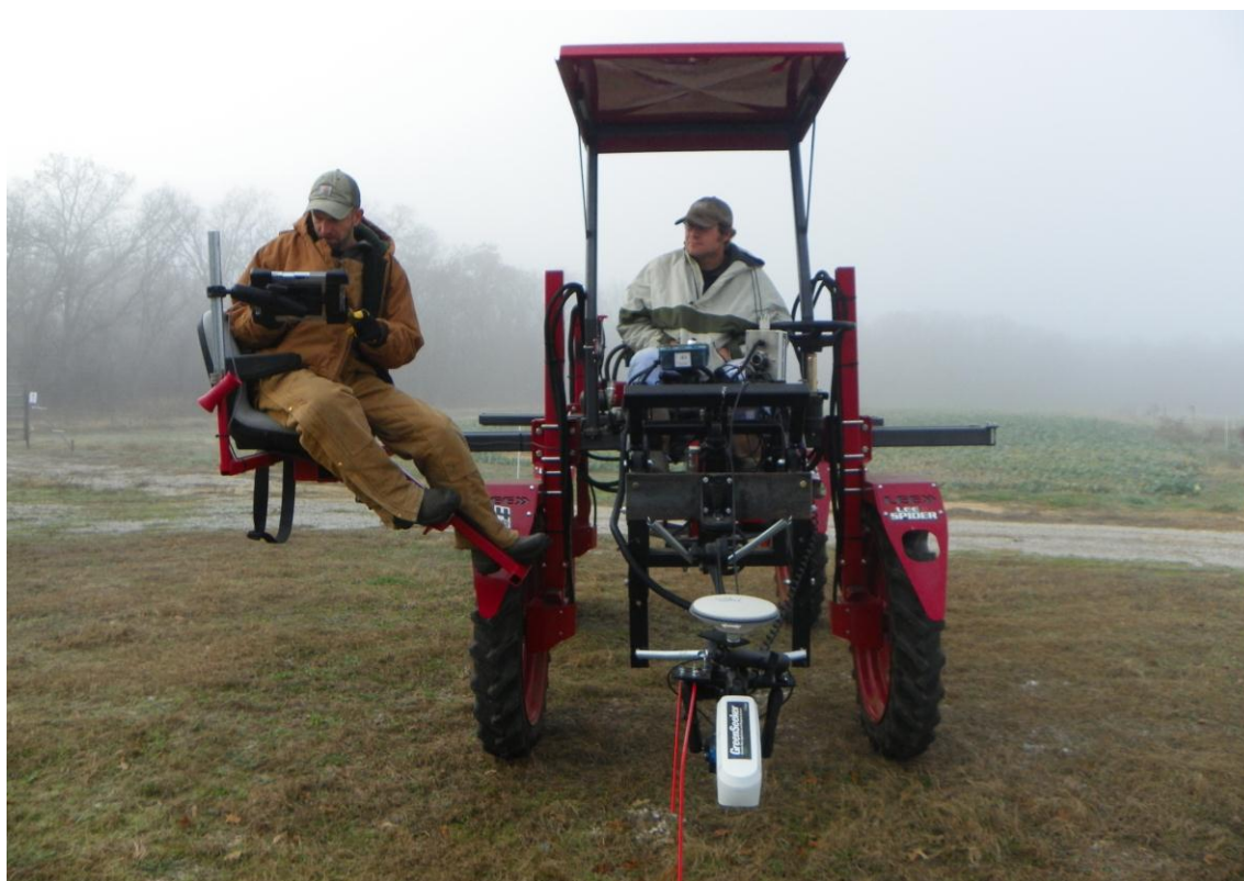
Figure 5. Spider used for transport of sensors across wheat experiments.
