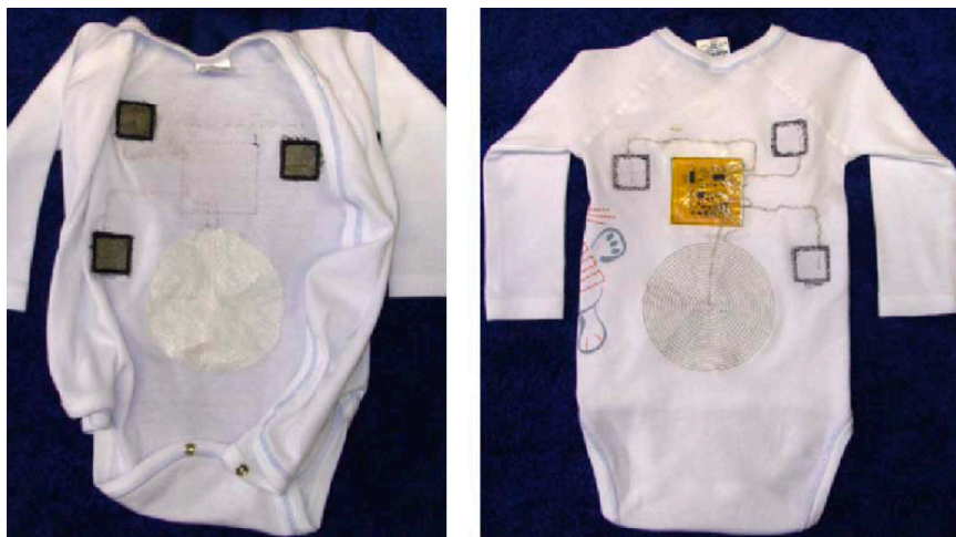
Figure 15. Baby suit prototype for ECG measurement. (Left) inside showing the Textrodes; (right) outside [31]. Copyright © 2005 Elsevier B.V.
