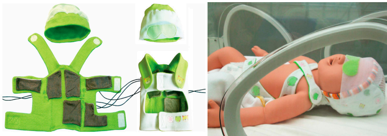
Figure 17. A prototype of the smart jacket ( left ) and a baby mannequin wearing the smart jacket inside the incubator ( right ) [11]. Copyright © 2009 IEEE
