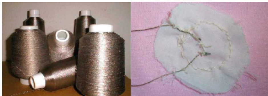
Figure 10. The conductive textile wires ( left ) and the connection of the sensor and the conductive wires ( right ) [10]. Copyright © 2010 Association for Computing Machinery, Inc.
