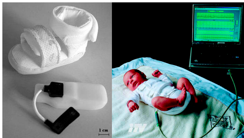
Figure 14. The BBA bootee ( left ) [9] Copyright © 2007 IEEE and the sensory baby vest ( right ) [12] Copyright © 2006 IEEE.
