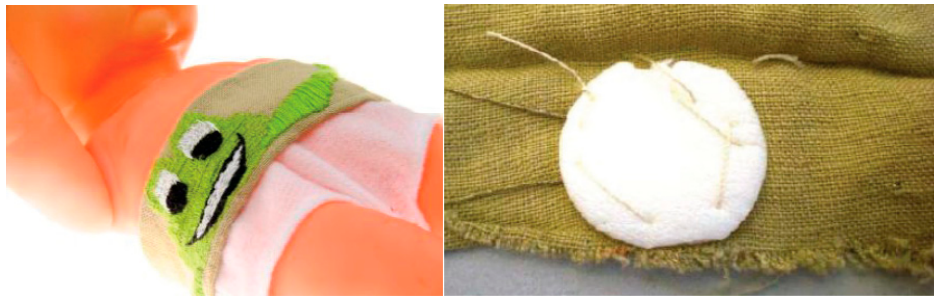
Figure 9. The prototype belt on a baby doll ( left ); and the isolation of the sensor in the belt ( right ) [10]. Copyright © 2010 Association for Computing Machinery, Inc.
