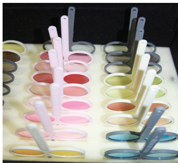
Fig. 1. MISViS filters consist of diverse colors of lenses. Each color family includes four to five lenses with differences in the degree of darkness.
