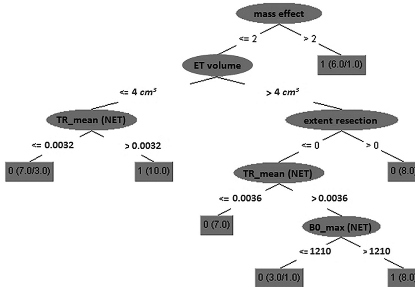
Fig 4. A 5-node decision tree calculated from all training data (no cross-validation). The numbers in each gray box indicate the predicted class label (0, survival time <18 months; 1, survival time >18 months), the total number of samples from both classes satisfying the conditions of each tree path, and the number of misclassified samples (shown only if nonzero). TR indicates trace intensity; BO_max indicates maximum BO intensity.
