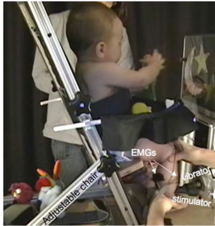
Fig. 1. Illustration of the infant reflex testing chair and stimulus apparatus. The configuration corresponds to the stimulation of the tibialis anterior muscle
