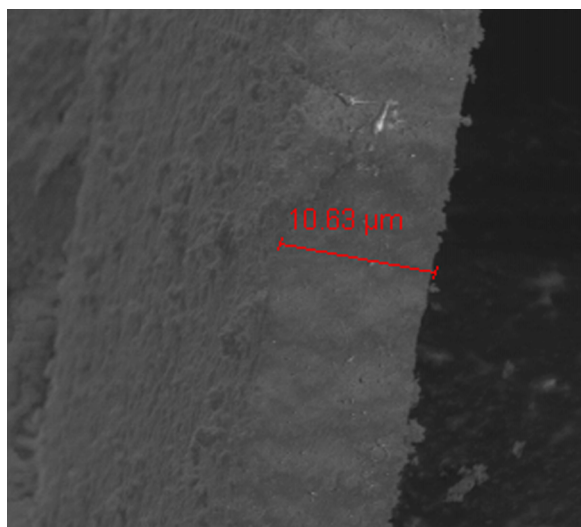
FIG. 3. SEM image highlighting the thickness of the sensor pellet fabricated from the emissive nanoscale scintillator. The pellet is shown here with the same relative orientation as it is depicted in Fig. 2.
