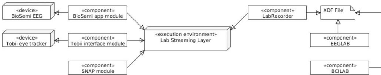
Fig 1. Experiment Software Architecture. The figure illustrates a conceptual overview of the software architecture used in the experiments. The BioSemi module provided a data stream containing the EEG data from the participant. The Tobii X2-30 module provided a data stream containing gaze and pupil diameter data of the participant. The SNAP module with custom scripts provided a data stream containing annotated stimulus events and markers. The Lab Streaming Layer collected and time synchronised all experimental data streams. The LabRecorder module recorded all data to file using the XDF format. Data analysis on the user study generated XDF files was carried out using the BCILAB and EEGLAB software libraries.
