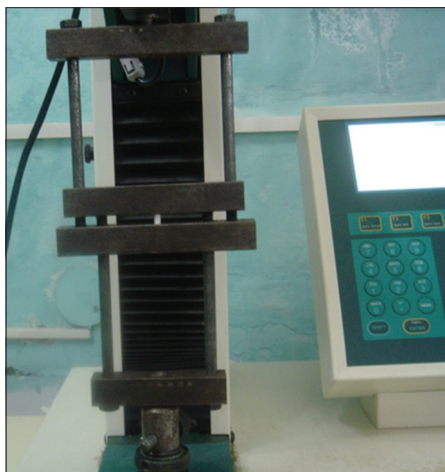
Figure 5: Specimen being tested for compressive strength.
