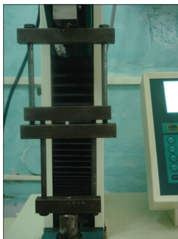
Figure 6: Specimen being tested for diametral tensile strength.
