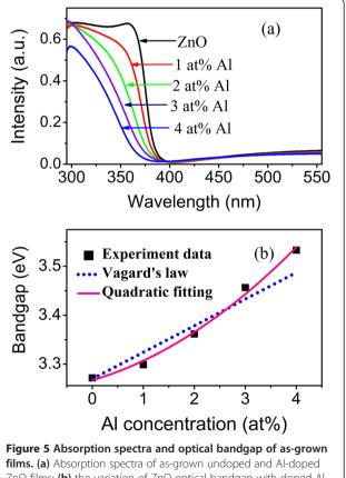
**films.** (a) Absorption spectra and optical bandgap of as-grown films. (b) the variation of ZnO optical bandgap with doped Al concentrations derived by Tauc's relationship, calculated by Vagard's law, and fitted by polynomial function.
