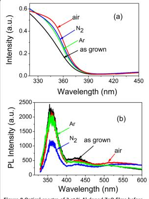
Figure 8 Optical spectra of 3 at.% Al-doped ZnO films before and after annealing. (a) Absorption spectra; (b) PL spectra of 3 at.% Al-doped ZnO films before and after annealing in Ar,  $N_2$ , and air ambient.
