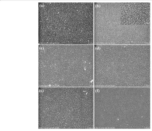
Figure 3 SEM images. (a) As-grown ZnO and (b) 3 at.% Al-doped ZnO films. High resolution images are also inserted; (c) undoped and (d) 3 at.% Al-doped films annealed in air; (e) undoped and (f) 3 at.% Al-doped ZnO film annealed in Ar.
