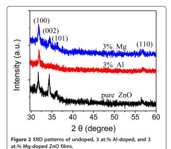
substrate surface and diffraction from (100) planes would be enhanced. Otherwise, it can also be seen from Figures 1 and 2 that the diffraction peak of (100) planes of doped films shifts to higher angle. This means that  $Zn^{2+}$  ions are replaced by  $Al^{3+}$  ions, resulting in the shrinkage of the lattice.
