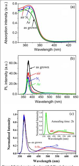
**Figure 7** Optical spectra of undoped ZnO films before and after annealing. (a) Absorption spectra; (b) PL spectra of undoped ZnO films before and after annealing in Ar,  $N_2$ , and air ambient; (c) normalized PL spectra of the undoped films after annealing in Ar for different times; normalized PL spectra annealed in Ar or air for 2 h are also inserted.
