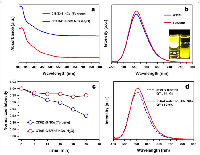
**Figure 5 Optical properties of CTAB-CIS/ZnS NCs. (a)** UV–vis absorption spectra and **(b)** PL spectra of CIS/ZnS NCs before (toluene dispersions) and after (aqueous dispersions) phase transfer using CTAB. Photograph of samples dispersed in different media under UV light is shown in the inset in the Figure 3b. **(c)** The evolution of PL intensity and **(d)** emission measurement after 6 months in the dark of CTAB-CIS/ZnS NCs.
