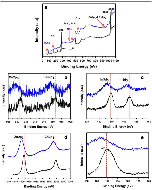
Figure 6 XPS spectra of the original (black lines) and CTAB-CIS/ZnS NCs (blue lines). (a) Survey spectra, (b) Cu 2p, (c) In 3d, (d) Zn 2p, and (e) S 2p.
