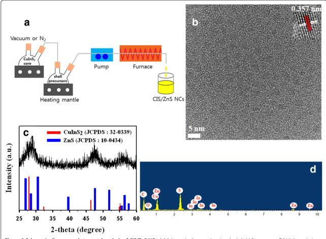
Figure 2 Schematic diagram and structural analysis of CIS/ZnS NCs. (a) Schematic diagram showing the hybrid flow reactor. (b) High-resolution TEM image of CIS/ZnS NCs. (c) X-ray diffraction pattern of CIS/ZnS NCs. (d) EDX spectrum of the CIS/ZnS NCs.
