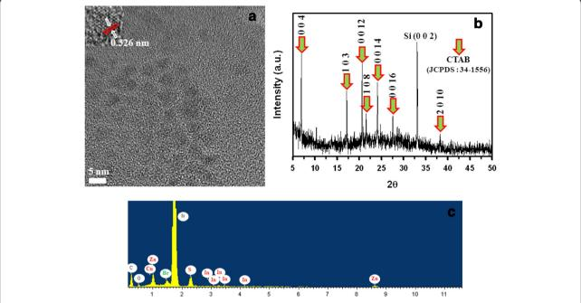
**Figure 4 Structural analysis of CTAB-CIS/ZnS NCs. (a)** High-resolution TEM image of CTAB-CIS/ZnS NCs. **(b)** X-ray diffraction pattern of CTAB-CIS/ZnS NCs. **(c)** EDX spectrum of the CTAB-CIS/ZnS NCs.
