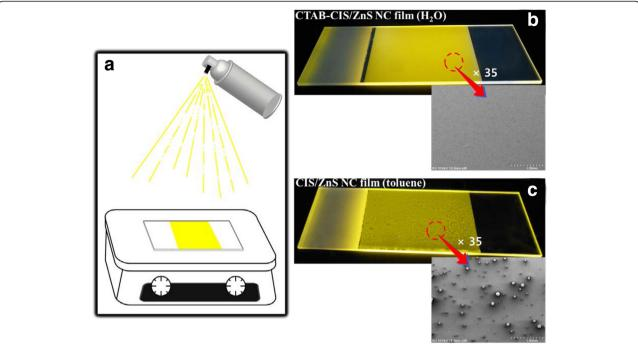
Figure 7 Spray process and photos of samples under irradiation of 254-nm light. (a) Scheme of spray process and photos of films coated on glass substrates; (b) CTAB-CIS/ZnS NC film (water) and (c) CIS/ZnS NC film (toluene).
