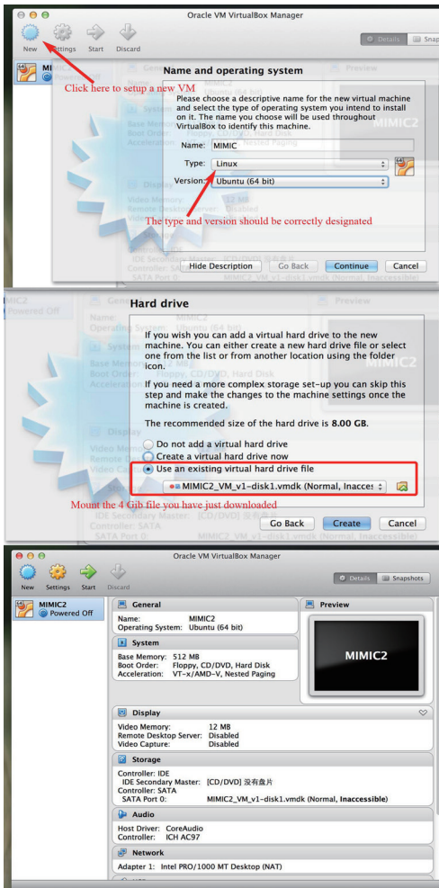
Figure 2 Setup of a virtual machine. MIMIC-2, multiparameter intelligent monitoring in intensive care-2.
