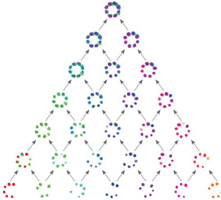
Figure 9. Illustration of a pyramid registration scheme. Pairs of particles are registered to each other and combined to form the next layer of the pyramid. The process is repeated until one particle remains which is the final average. This procedure scales quadratically with the number of particles.
