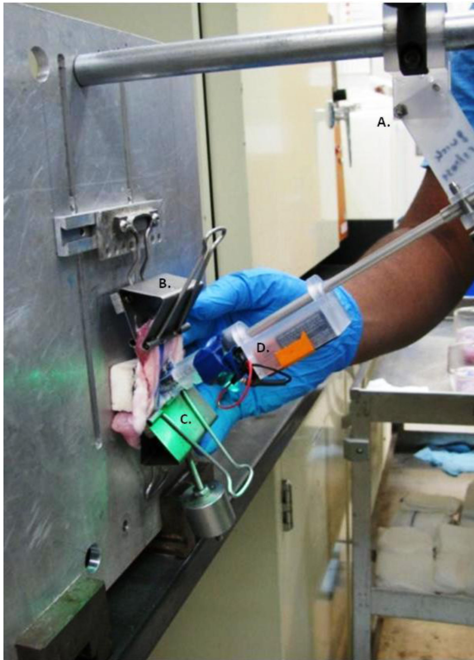
Figure 2. Mesh fixation apparatus. Mesh fixation devices were oriented at specific angles to the tissue using a bracket that fixed the shaft at the desired angle (A). The abdominal wall specimen was fixed superiorly to a clip attached to the metal backing plate (B), and inferiorly to a 168 g weight providing tension equal to an insufflated abdominal wall (C). The tip of the mechanical fixation device was attached to a preload force measuring device to ensure that constructs were applied with a preload force between 1.25 and 1.90 lbs (D).
